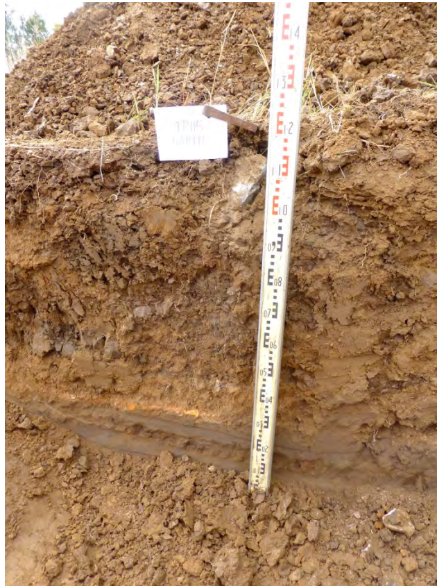
Plate 13: Interface between general fill and natural alluvium, TP115
