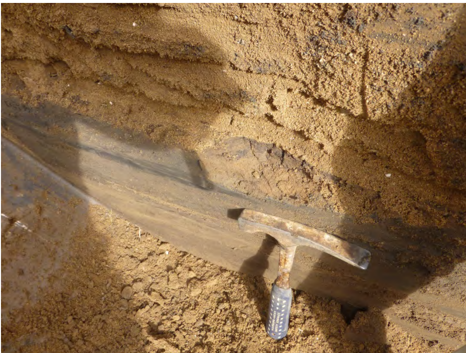
Photograph D49 – TP117 – Detail contact coarse sand layer.
