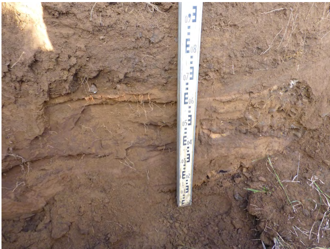
Plate 17: Faint layering within alluvial silty SAND, TP109
