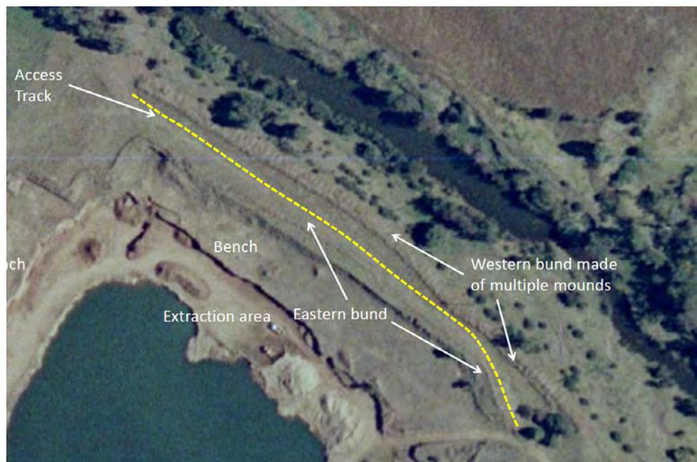
Plate 32b: Enlargement of 2001 air photo showing western levee – note multiple mounds of earth on west side of access track
