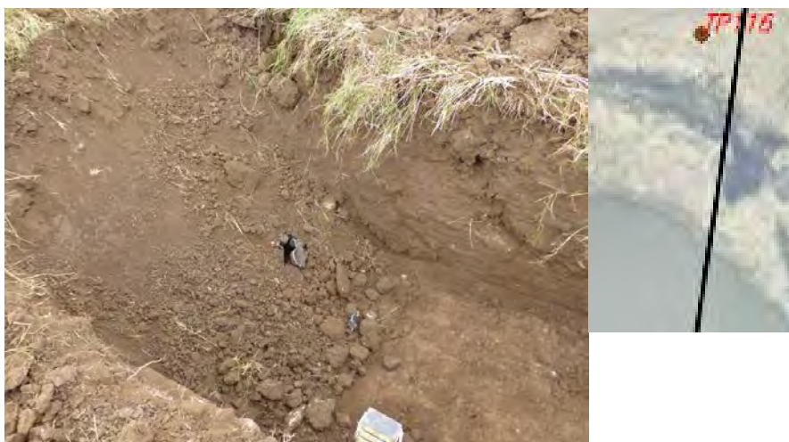
Plate 16: Fill material adjacent to main breach backfill area, TP116
