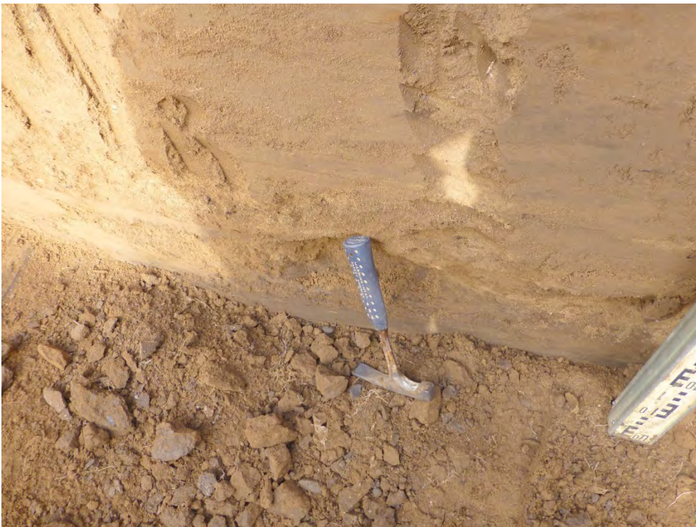
Photograph D51 – TP118 – Details of contact coarse sand.
