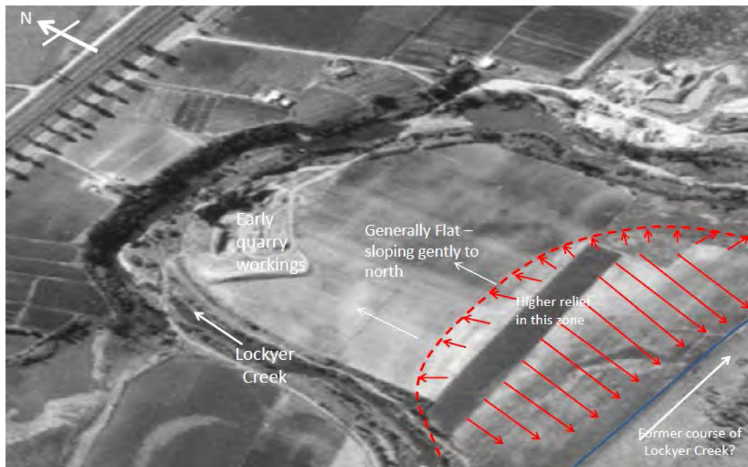
Plate 19: Oblique view generated from 1982 air photo showing relief interpreted from stereoscope
